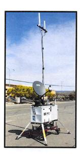
The CRD™ for FirstNet is a <u>Customer-Owned</u> AT&T FirstNet deployable cell tower. It generates an area of FirstNet Cellular and Wi-Fi Internet coverage, anywhere, anytime. Your very own Cell-On-Wheels (COW) can be deployed by a single person, within minutes, wherever needed. Never go without Internet and Cell service again!
